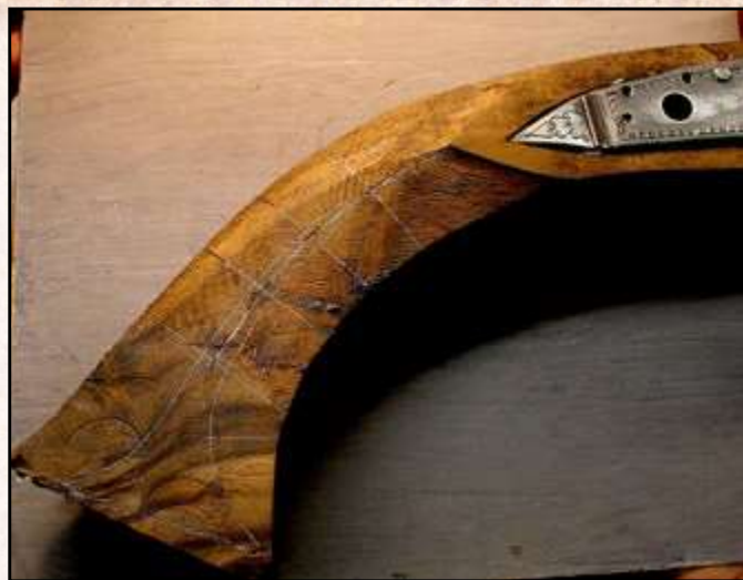
Fig. 6. The centerline of this pistol butt was drawn using a dial caliper and a French curve. Note the thin triangular section that must be removed from the bottom to allow alignment of the template with the centerline of the butt.
