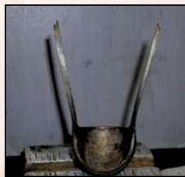
Fig. 7. You'll know if your brass is sufficiently annealed if you can easily spread the tangs by gentle hand pressure against a round surface.
