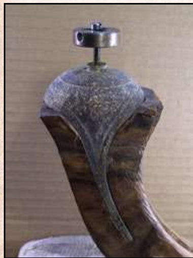
Fig. 18. Sometime as the butt approaches final fit all around, your inletting is so good that you can't get the butt cap out. This improvised handle might just do the trick. It that won't budge it, run the machine screw down against the wood and carefully back the cap out.
