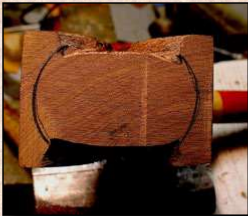
Fig. 13. The circumference of the cap has been penciled on the butt flat as a guide, but follow your black around the oval as you continue inleting.
