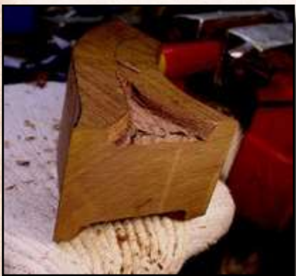
Fig. 10. Read your inletting black to tell you where to remove wood. This is a slow repetitive process. Patient persistence is the key to success.
