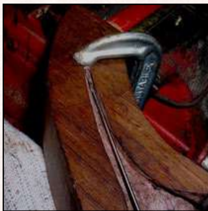
Fig. 16. A 1/16" bit with a long shank can drill a relief for the spiked hold-down tabs at the ends of the tangs.
