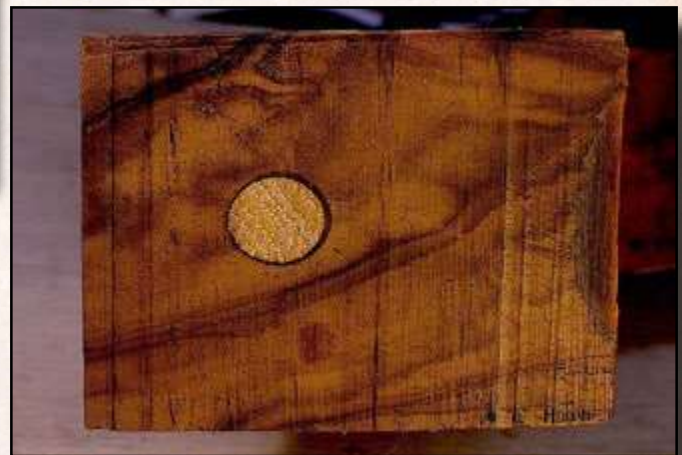
Fig. 2. This reinforcement method has been used on two rifles with broken wrists. I put a 1/2" dowel in one and a length of 1/4" all-thread rod in the other. Very sturdy, doesn't show, and is prettier than a metal patch.
