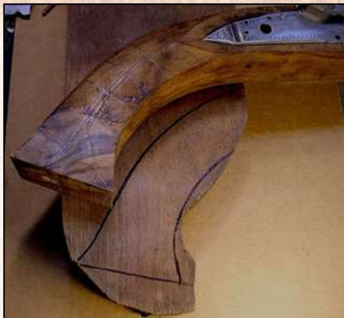
Fig. 3. The profile of my pistol butt was traced onto another piece of walnut.
