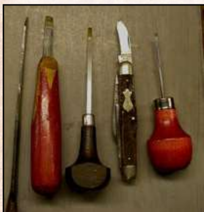
Fig. 9. These tools (from left) are a deep mortise chisel, a homemade paring chisel, a chisel made from a 1/8" diameter lathe cutter blank in a commercial handle (see suppliers), Dad's pocket knife with a re-ground blade and a 3/32" offset chisel.
