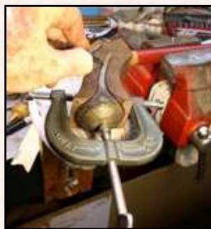
Fig. 11. As the rim of the cap nears the butt flat, apply gentle pressure via a three-pad edging clamp.
