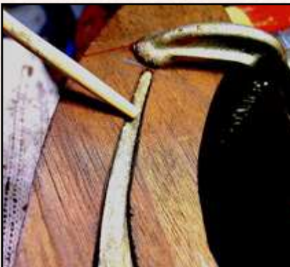
Fig. 17. This tang is now secured by the spiked hold-down tab. There is a lot of blackened dirty wood standing proud of the tang surface that must be removed.
