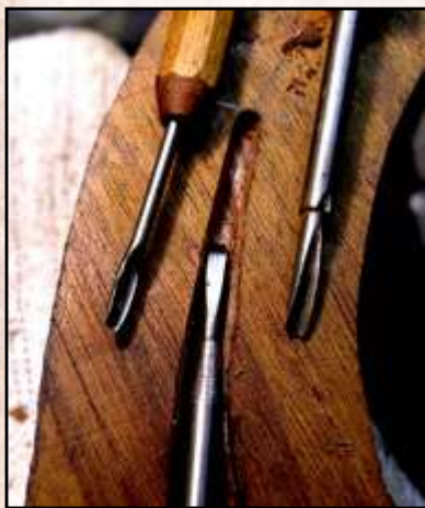
Fig. 14. As the tang inlets grow progressively thinner, your tools must be smaller. Custom gouges and chisels can be ground from "1/8" thick drill rod or lathe cutter blanks.
